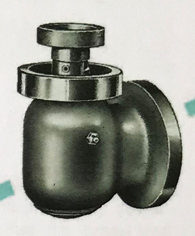
The vertical milling head swivels  $90^{\circ}$  left and right. A graduated scale clearly shows the desired angle setting.
