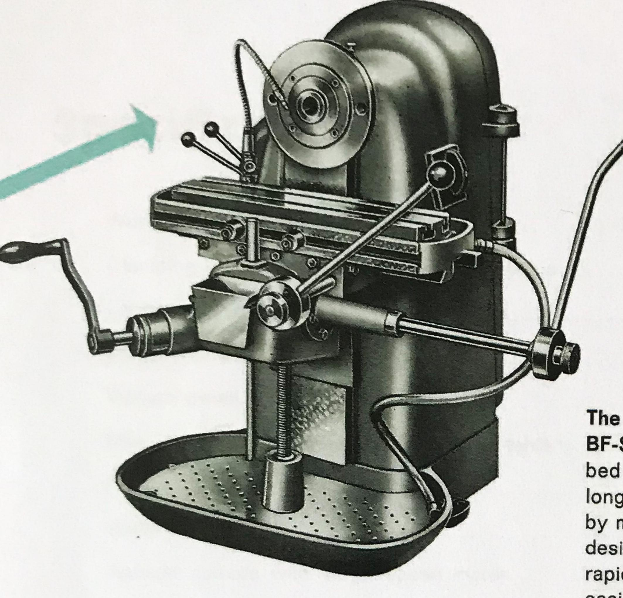
With lever control, accurate and rapid table movements are obtained.
